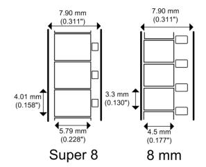
**The Fuji Single 8** has the same width and sprocket dimensions as Super 8, but is thinner film. Therefore the running times, for the same diameter spools will be longer, as more film will fit into the same space on the reel. Reel which can hold 120 meters of Super 8 will hold 180 meters of Single 8 film.
